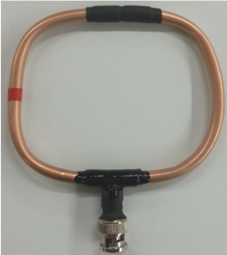
Actual size of the Loop Antenna BNC Connector Usable from 1Mhz to 800Mhz
